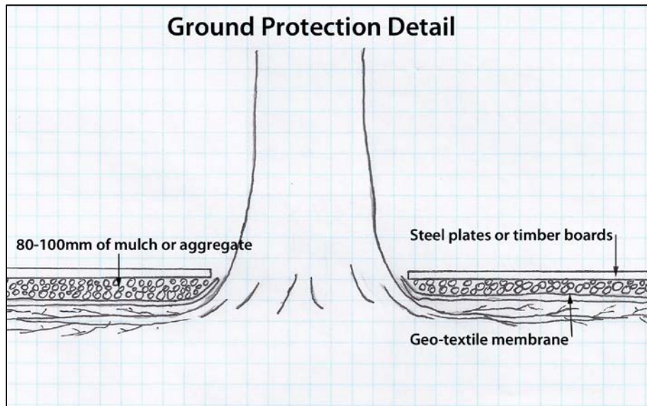
Figure B: Specification of appropriate ground protection –To be used where construction access passes within the TPZ of Trees 1, 2 and 3.
